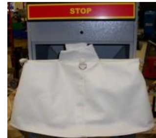
3. Ensure textile hanger & retaining clip are inline
