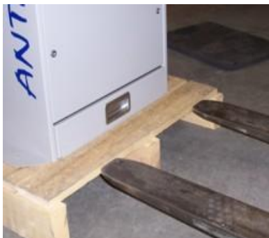
3. Position Fork Lift extensions in-line with the pallet top.
