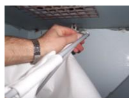
5. Remove rear retaining clip
