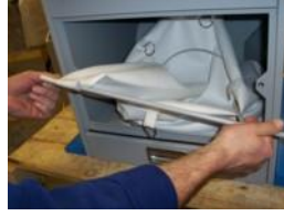
8. Remove shaker frame from dust bag
