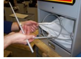
9. Remove shaker frame from extractor
