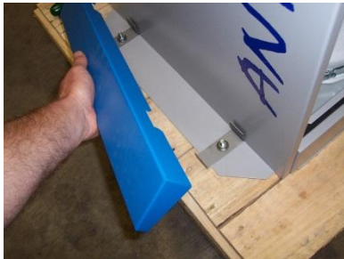
1. Remove the two base covers to expose transit bolts.
