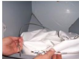
11. Remove retaining clip from extractor
