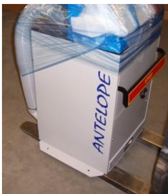
5. With the machine sat stable on the Fork Lift extensions – lower to the ground.
