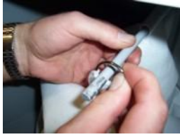
7. Remove front retaining clip
