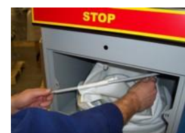
6. Remove shaker frame from extractor
