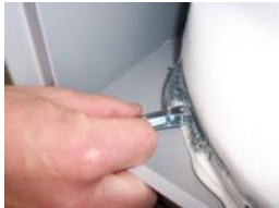
10. Release snap over retaining clip
