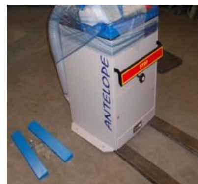
6. Slide the machine off the Fork Lift extensions onto the ground.
