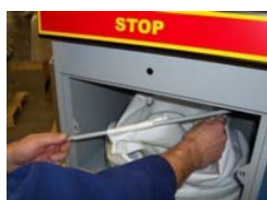
6) Remove shaker frame from extractor
