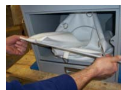
8) Remove shaker frame from dust bag
