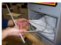
9) Remove shaker frame from extractor
