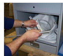
5) Re assemble shaker frame & orientate textile hanger front to back
