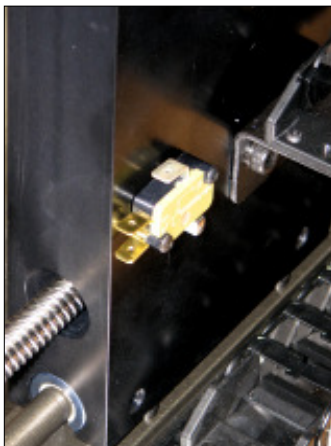
X Axis Switch located behind rear column
