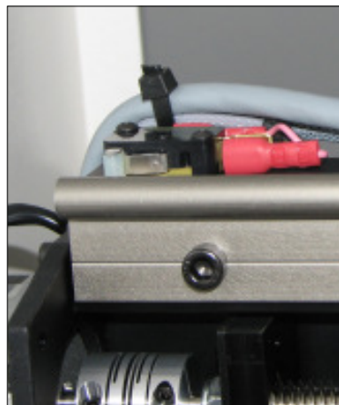
Y Axis Switch located top rear corner of crossbeam
