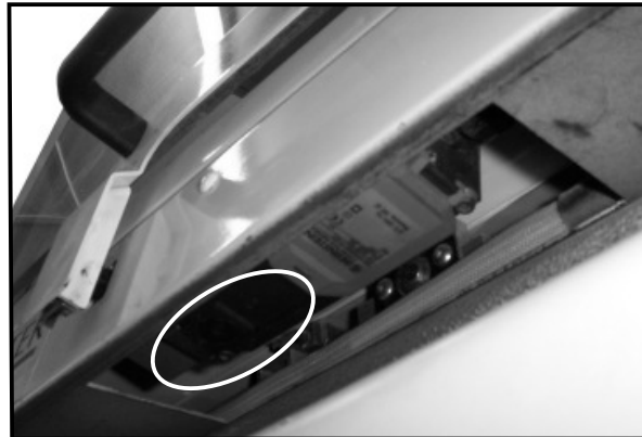
Left: The interlock guard switch unit (circled) is located behind the lower front machine panel.
