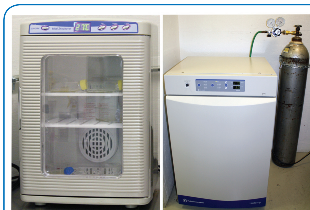
Figure 2: Cell culture incubators for standard or controlled atmospheric conditions.
