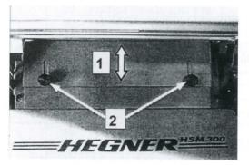
When adjusting swivelling table the cover sheet (1) needs to be adjusted.
