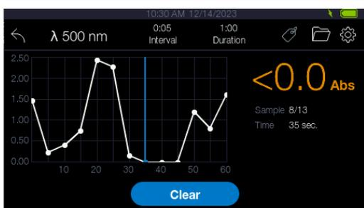
14. If the measured values from the sample fall outside of the photometric range, the absorbance value will report in orange colour either <0.0A if the measurement is below 0A or >2.6A if the measurement is above 2.6A
