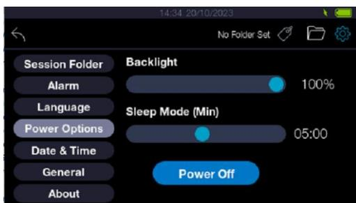
1. This section allows the user to set the level of backlighting for the display. Please note that applying more backlighting will drain more power from the battery and therefore may deplete it quicker.
