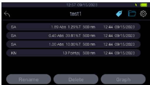
3. Saved measurements will be recorded in the folder. The first column indicates the type of measurement. SA stands for "sample," KN stands for "kinetics".
