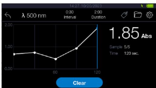
12. After all the measurements are done, the graph will be displayed, showing each data points. Click on the data points to display the Absorbance or T% value associated to it, as well as the time stamp.
