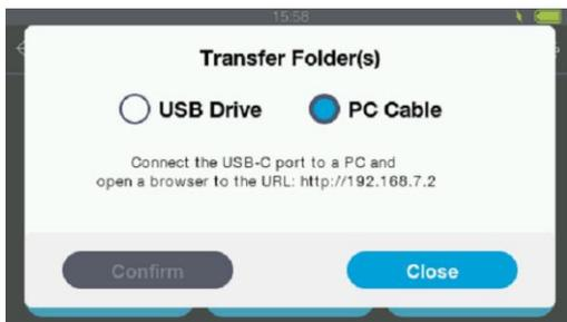
4. Select "PC Cable" then open a Web browser page and enter the URL specified on the device in the address bar.
