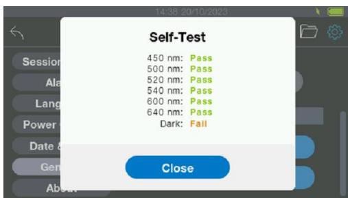
8. Press the “Self-Test” function to run a diagnostic of the hardware. The device will return the results of the test. If a parameter fails, it will be displayed in orange.
