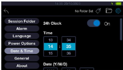
1. This section allows the user to set the time, time format, date and date format as required.
