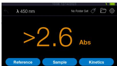
Multiple samples can be compared with the same reference by placing different samples in the cuvette holder and making measurements for each one by pressing the “sample” button.
