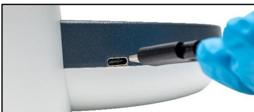
USB-C port for connecting to PC/laptop and charging the device, using the USB-C cable supplied.
