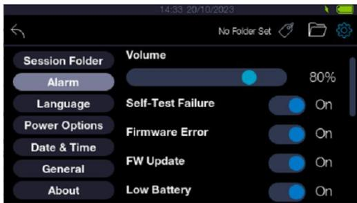
1. This section allows the user to enable/disable various alarms on the unit. Toggle the alarm ON or OFF according to your preference for each of the features displayed.
