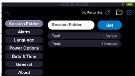
5. If you do not wish to save measurements, delete the folder name in the white box and press "Set." "No Folder Set" will be indicated near the tag icon to indicate that subsequent measurements will not be saved.
