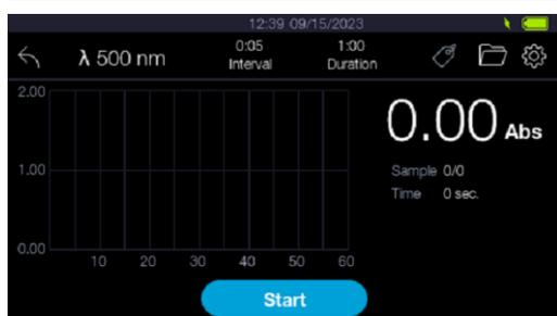
7. Press "Interval" or "Duration" on the top of the screen to set the time between measurements and the total duration of the assay.
