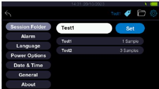
1. This section allows the user to create new folders or select existing folders that will be used to store sample results.
