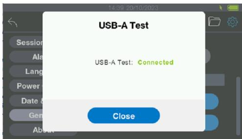
9. Press the “USB-A Test” button to test the connectivity with a USB flash drive. The instrument will report whether the connectivity is established with an external flash drive.
