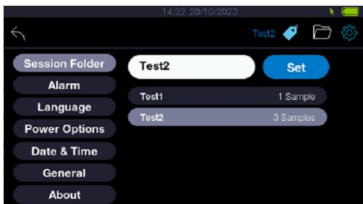
4. To use an existing folder to save data, highlight the folder and press "Set." In this example, "test2" becomes the active folder and is displayed next to the blue tag. All subsequent measurements will be saved in this folder.
