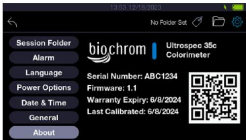
1. This section displays the serial number of the unit and gives information about firmware version, warranty expiry and last calibration date.
